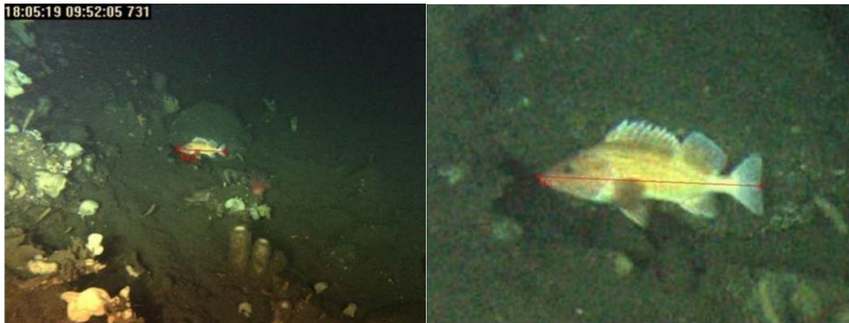
Figure 14.10table.—Yelloweye rockfish with a 3D point (red circle) and a total length (red line) measured in the stereo camera overlapping field of view in the SeaGIS EventMeasure software.
